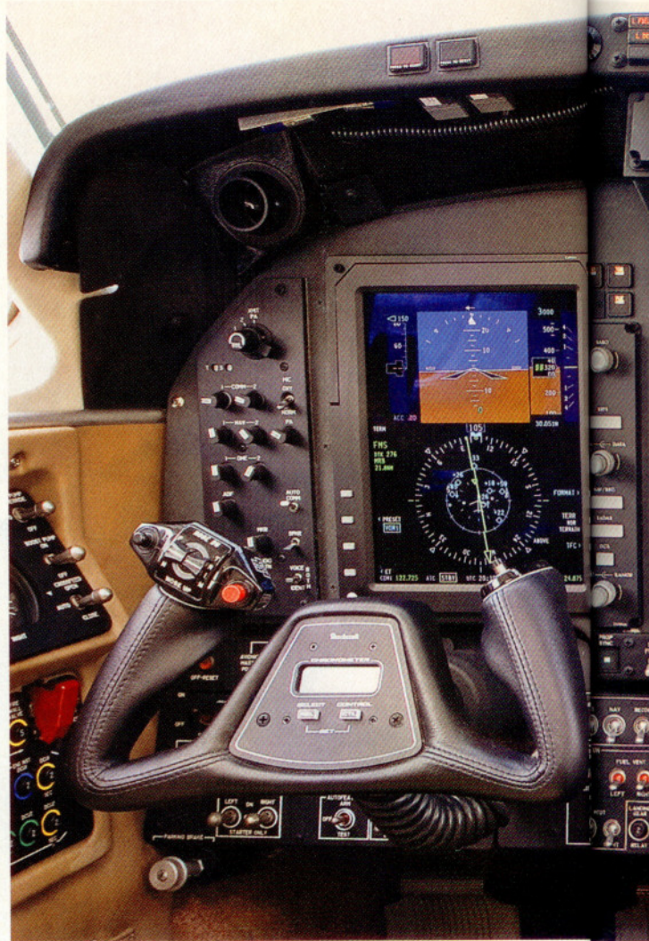
The C90GTi cockpit is a mix of old and new. The power levers, pressurization gauges, and trim controls are in the same places as before (left), but the Pro Line 21's FMS occupies space previously assigned to autopilot controls. Buttons at the bottom right of the photo are for calling up electronic chart views on the multifunction display. Not shown is a hinged cover that can be lowered over the center pedestal—to protect its hardware from being kicked by ingress and egressing pilots.
